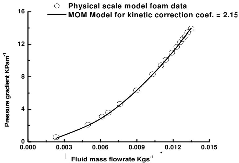
Figure 3. Graph of pressure gradient vs. fluid flow rate in a physical scale model foam sample, for the calibration of the MOM model. Reynolds number is from 148 to 890.
