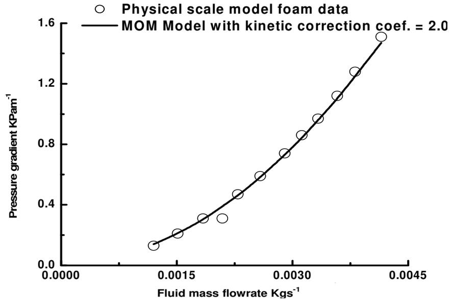
Figure 4. Graph of pressure gradient vs. fluid flow rate in a physical scale model foam sample, for the calibration of the MOM model. Reynolds number is from 86 to 269.
