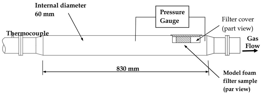
Figure 2. Schematic diagram of a flow rig model foam sample holder.
