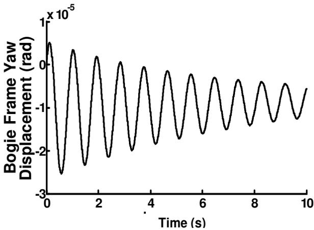
Figure 15. Dynamic response of railway carriage bogie frame to yaw displacement at forward railway carriage velocity (76 Km/h).
