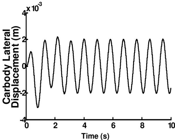
Figure 4. Dynamic response of railway carriage carbody to lateral displacement at critical hunting velocity (76 Km/h).
