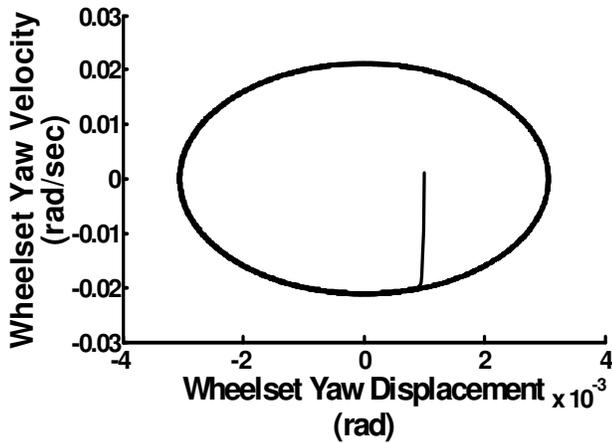
**Figure 8.** Phase portrait trajectories of wheelset dynamic response to yaw displacement at critical hunting velocity (76 km/h).
