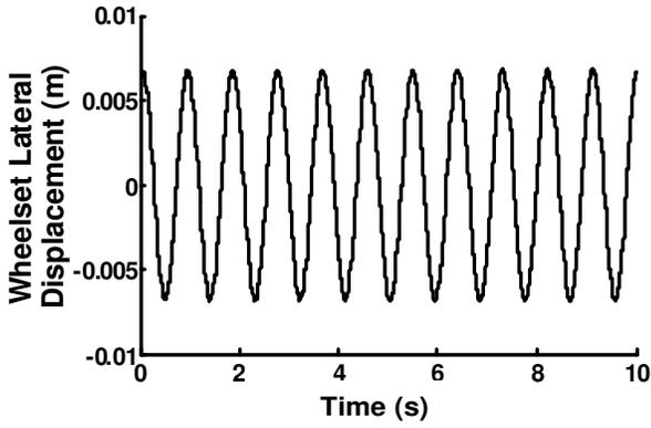
Figure 2. Dynamic response of railway carriage wheelset to lateral displacement at critical hunting velocity (76 Km/h).
