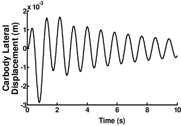
Figure 14. Dynamic response of railway carriage wheelset to yaw displacement at forward railway carriage velocity (76 Km/h).
