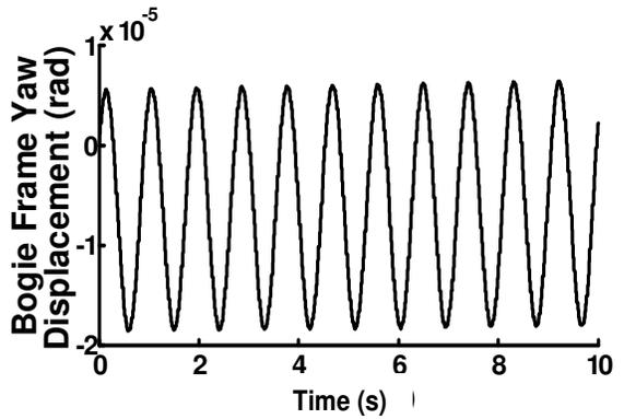
Figure 6. Dynamic response of railway carriage bogie frame to yaw displacement at critical hunting velocity (76 Km/h).
