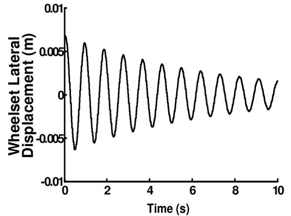
**Figure 11.** Dynamic response of railway carriage wheelset to lateral displacement at forward railway carriage velocity (76 Km/h).
