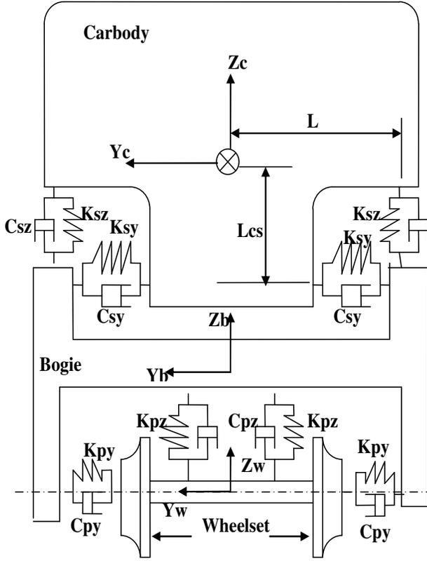
**Figure 1.** Front view of railway carriage components equipped with sets of primary.
