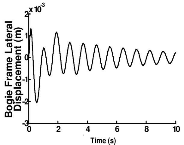
**Figure 12.** Dynamic response of railway carriage bogie frame to lateral displacement at forward railway carriage velocity (76 Km/h).
