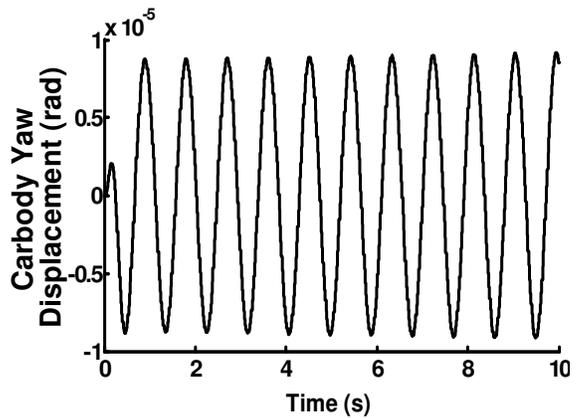
Figure 7. Dynamic response of railway carriage carbody to yaw displacement at critical hunting velocity (76 Km/h).
