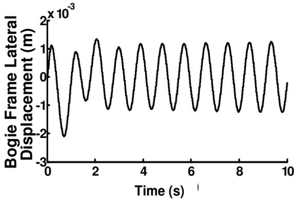
Figure 3. Dynamic response of railway carriage bogie frame to lateral displacement at critical hunting velocity (76 Km/h).
