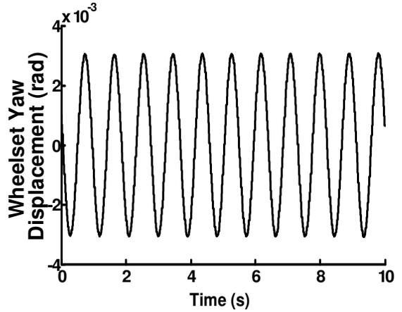
Figure 5. Dynamic response of railway carriage wheelset to Yaw displacement at critical hunting velocity (76 Km/h).
