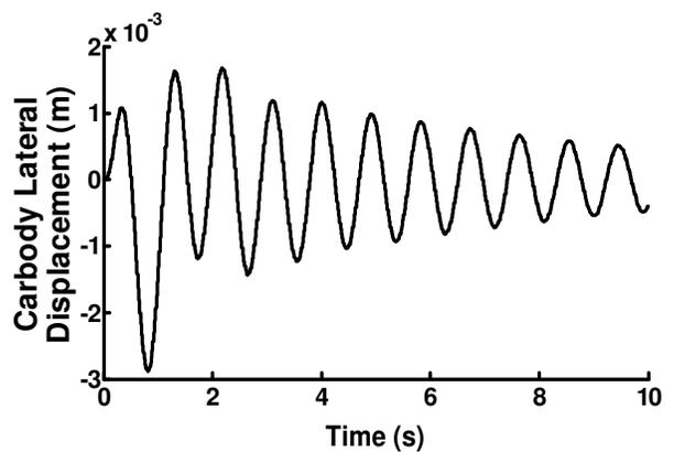
**Figure 13.** Dynamic response of railway carriage carbody to lateral displacement at forward railway carriage velocity (76 Km/h).
