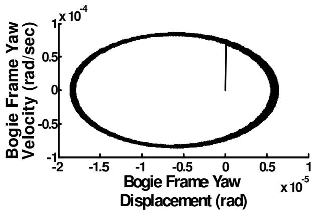
**Figure 9.** Phase portrait trajectories of bogie frame dynamic response to yaw displacement at critical hunting velocity (76 km/h).
