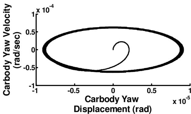
**Figure 10.** Phase portrait trajectories of carbody dynamic response to yaw displacement at critical hunting velocity (76 km/h).
