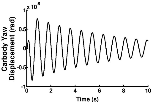
Figure 16. Dynamic response of railway carriage carbody to yaw displacement at forward railway carriage velocity (76 Km/h).
