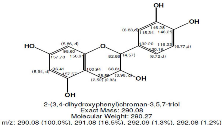
**Figure 2.** Structure of catechin showing <sup>1</sup>H and <sup>13</sup>C chemical shifts as elucidated using NMR, 500MHz
