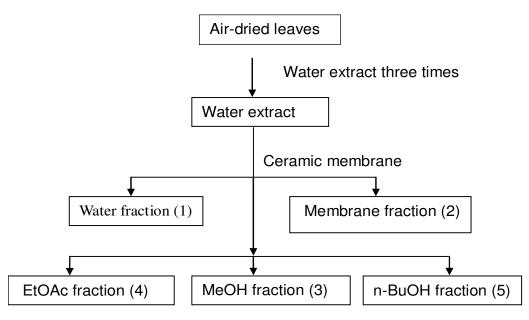
Figure 1. The chart of extraction process.
