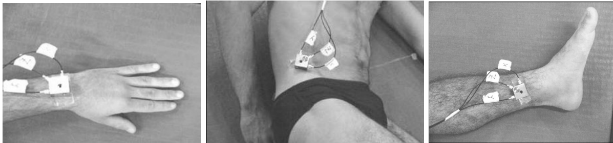
Figure 1. Accelerometer settling at the judokas wrist, hip and ankle, according to the method adopted by Santos (2003). Source: Santos (2003: 45).
