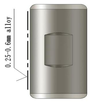
Figure 2. Coupling with circular arc and coating with alloy.
