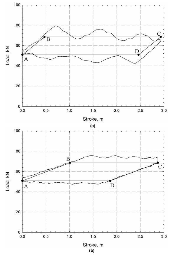
Figure 3. Dynamometer card of Well L1-48 without anchoring for (a) N80 tubing and (b) FRP tubing.
