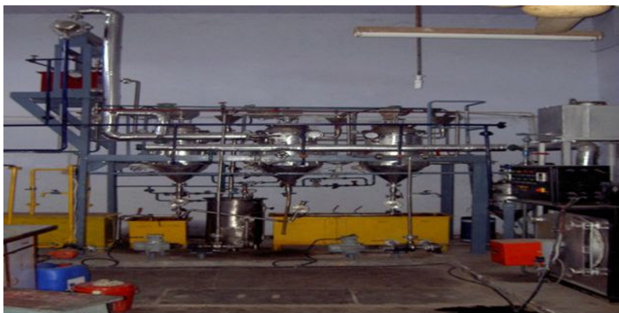
Figure 3b. Photograph of Pilot Plant used for Biodiesel production.
