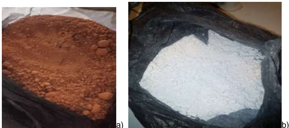
Figure 4. Partial view of: a) red and b) white locally available inert dusts.
