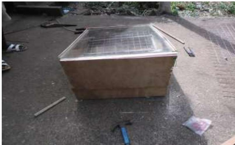
**Figure 6.** Cabinet style dryer with glass top.
