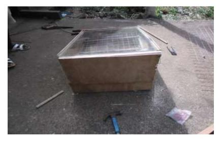
Figure 6. Cabinet style dryer with glass top.
