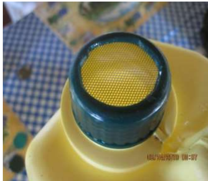
Figure 3. Modified (ventilated) container cap.
