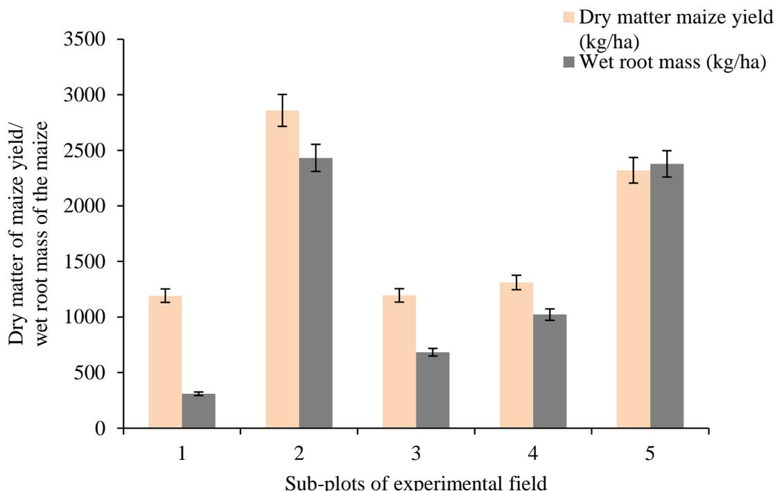
**Figure 5.** Dry matter of maize yield and wet root mass of the maize crops at various levels of tractor compaction treatments on different experimental sub-plots.
