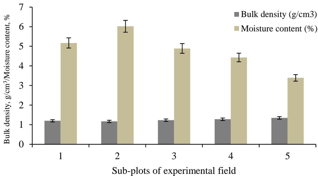
**Figure 2.** Effects of compaction treatments on the soil bulk density and moisture content of the different sub-plots.
