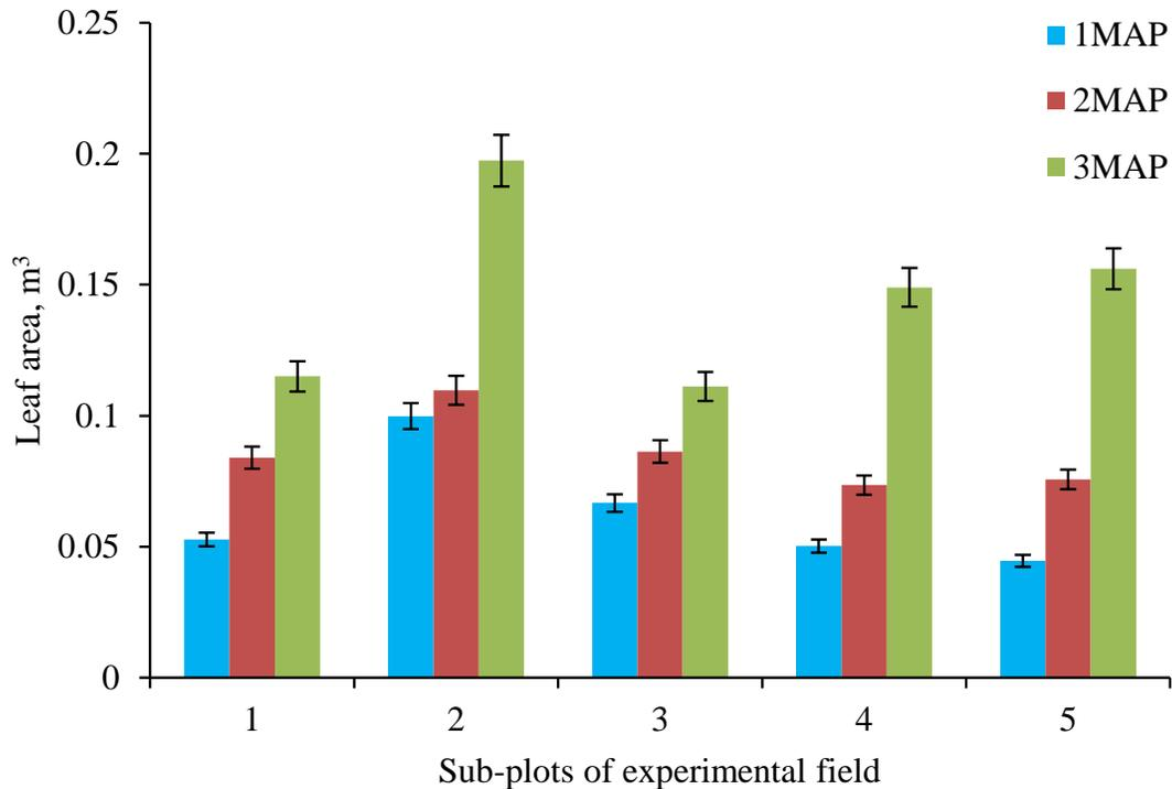
**Figure 4.** Variation of maize plant leaf area with the number of months after planting at various levels of tractor compaction treatment for the different sub-plots (MAP = Months After Planting).
