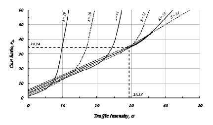
Figure 7. Determination of optimum number of berths, o, Alexandria port, case study.
