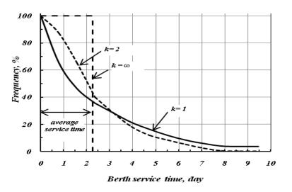
Figure 3. Service time distribution as Erlang Function, hypothetical port.
