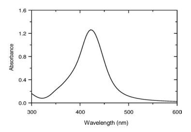
**Figure 1.** UV-Vis absorption spectra of biological biosynthesized silver nanoparticles from Onion extract.
