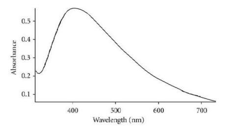
**Figure 2.** UV-Vis absorption spectra of chemically synthesized silver nanoparticles from sliver nitrates.
