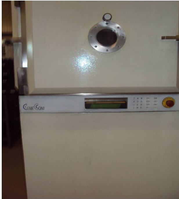
Figure 2. PVD apparatus used in the experiments.
