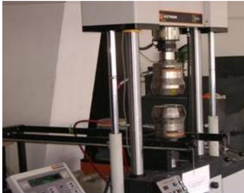
Figure 4. Instron 8501 dynamic test device.
