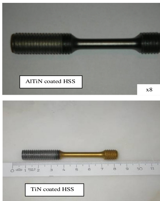
Figure 3. HSS sample coated with PVD.
