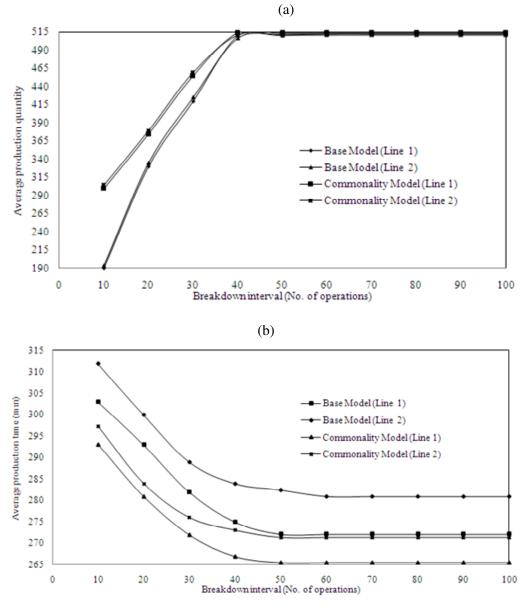
**Figure 5.** (a) Effect of machine breakdown on (a) production quantity and (b) cycle time when the number of sub-components is 60 and lead time is zero (Case-2).
