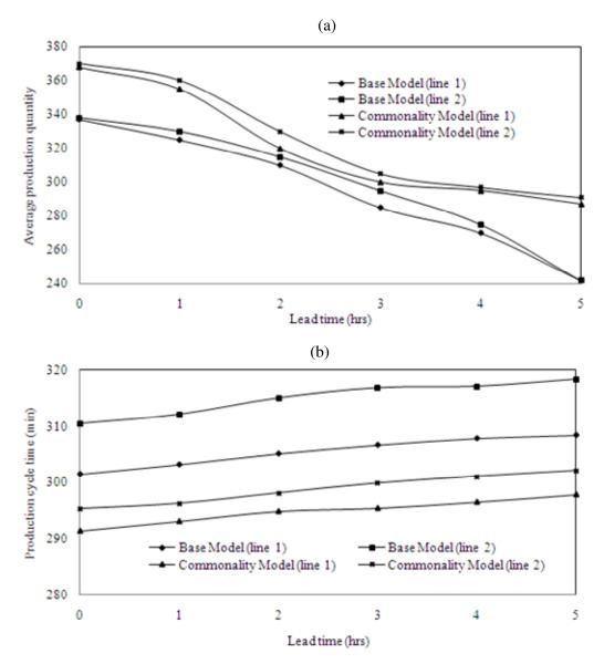
**Figure 7.** (a) Throughput quantity and (b) average time for base and commonality models for Case-4, when the number of parts is 60 units.
