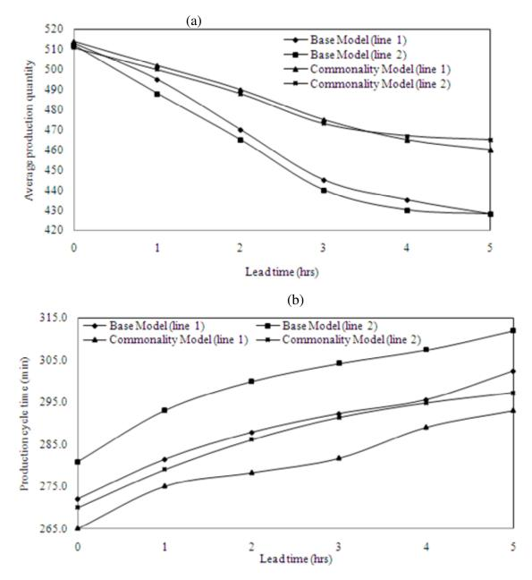
**Figure 6.** (a) Throughput quantity and (b) average time for base and commonality models for Case-3 when the number of parts is constant at 60 units.
