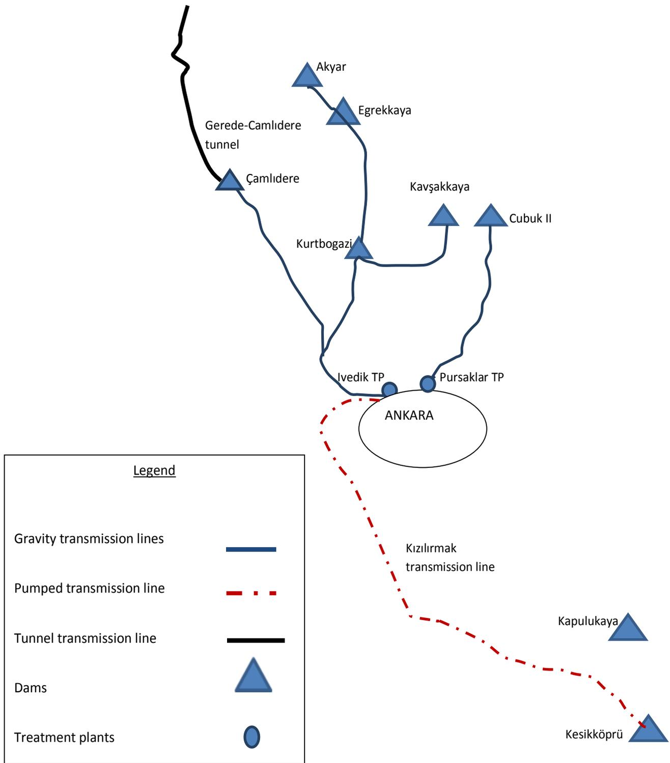
**Figure 5.** Schematic map of Ankara's dams and transmission lines (Gravity transmission lines are in service at present, pumped transmission line used during drought and tunnel is under construction).
