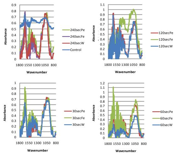
Figure 1. FTIR spectroscopy of corona treated paper samples.
