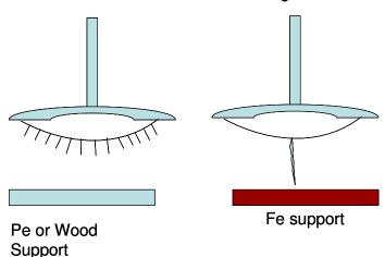
**Figure 3.** Nature of glow discharge and electrical sparc on different support media.
