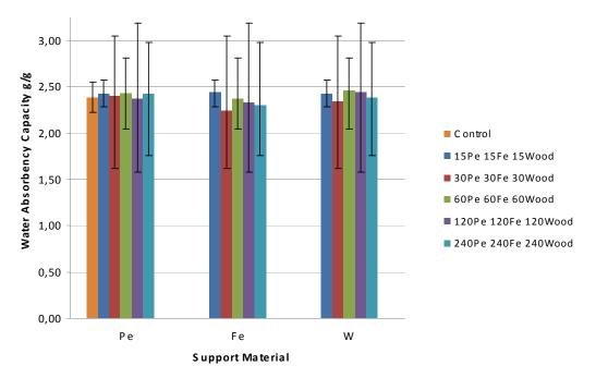
Figure 4. Absorbency of paper products on different treatment period and support media.
