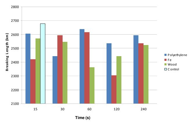
Figure 2. Breaking length of the paper samples in different treatment period and support media.
