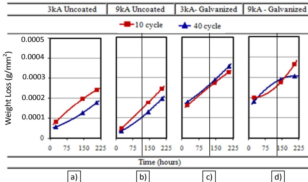
**Figure 5.** Change of weight loss in the welded specimens of the galvanized and uncoated steels.
