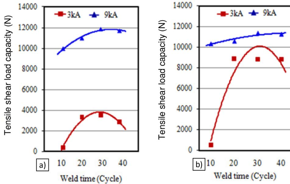
**Figure 4.** Tensile shear load capacities of the welded specimens. a) galvanized specimen, b) uncoated specimen.
