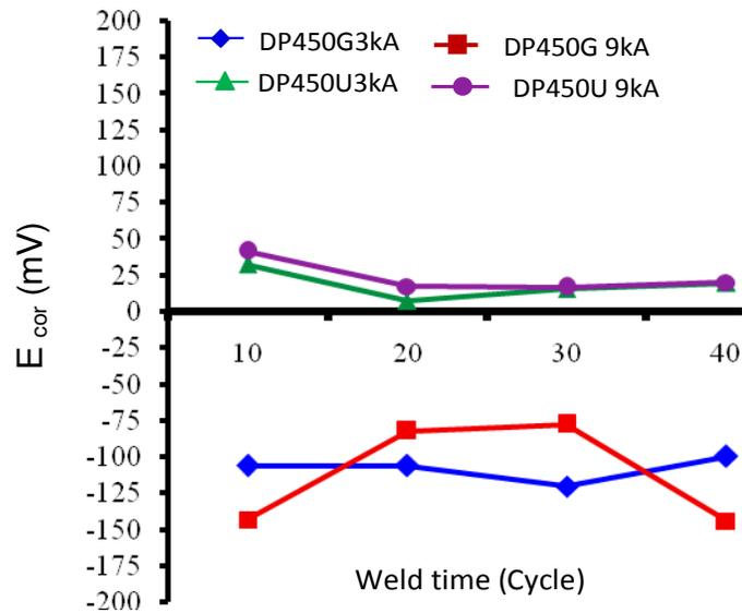
**Figure 7.**  $E_{cor}$  values of the welded specimens of the galvanised and uncoated steels.
