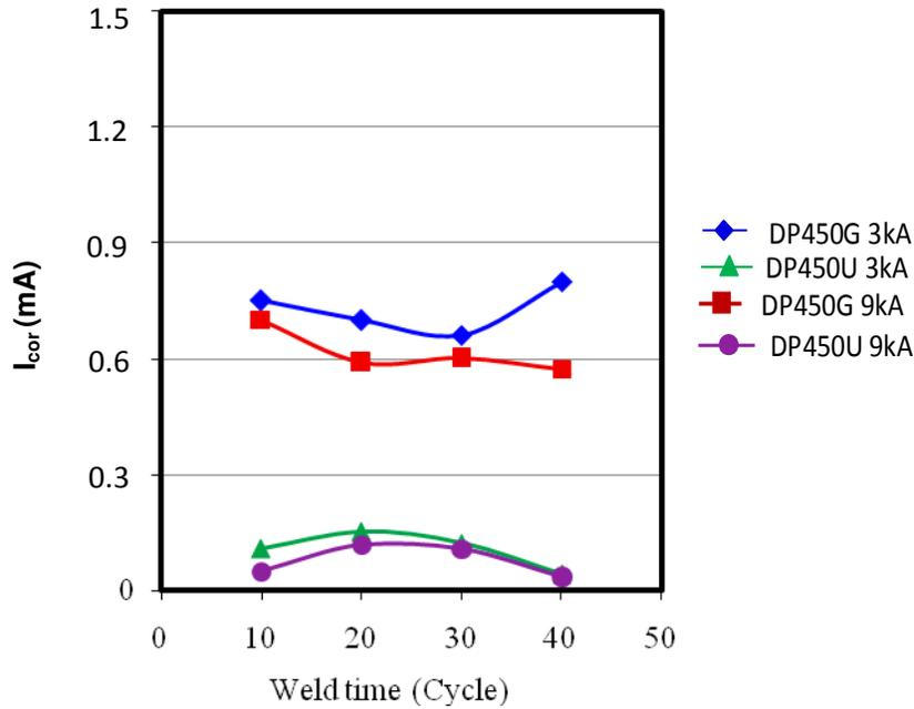
**Figure 6.**  $I_{cor}$  values of the welded specimens of the galvanised and uncoated steels.
