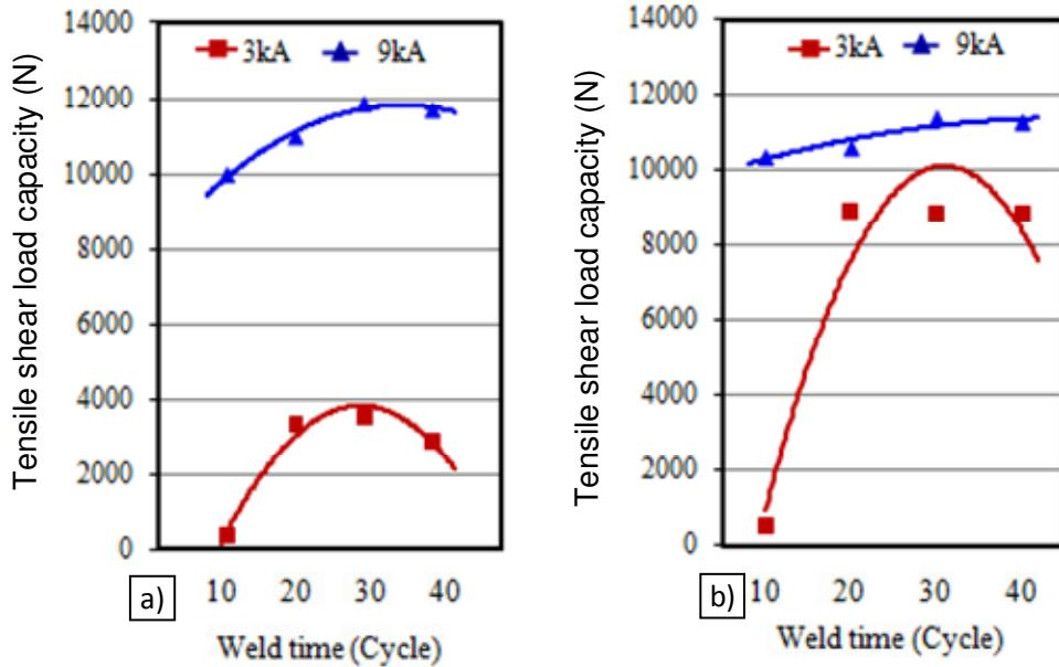
**Figure 4.** Tensile shear load capacities of the welded specimens. a) galvanised specimen, b) uncoated specimen.
