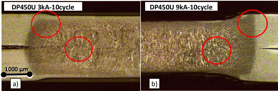
**Figure 1.** DP450U (a) 3kA-10c and (b) 9kA-10c macrostructure of spot welding.
