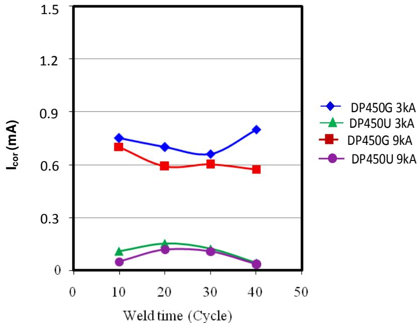
**Figure 6.**  $I_{\text{cor}}$  values of the welded specimens of the galvanised and uncoated steels.
