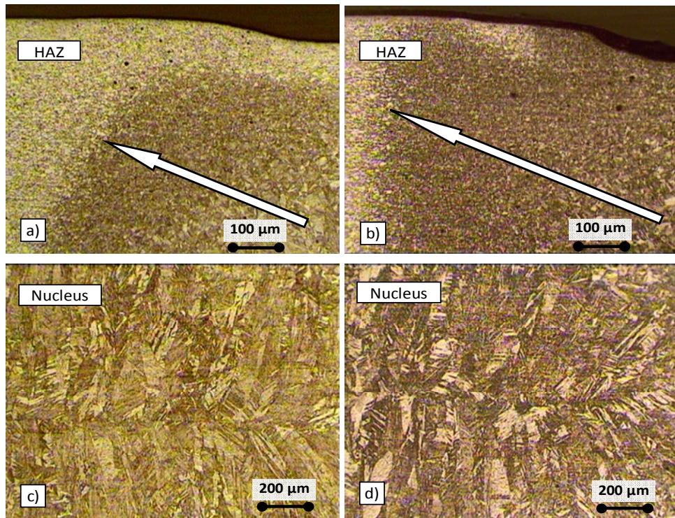
**Figure 2.** DP450U 3kA-10c (a: HAZ, c: nucleus) and 9kA-10c (b: HAZ, d: nucleus) microstructure of spot welding.
