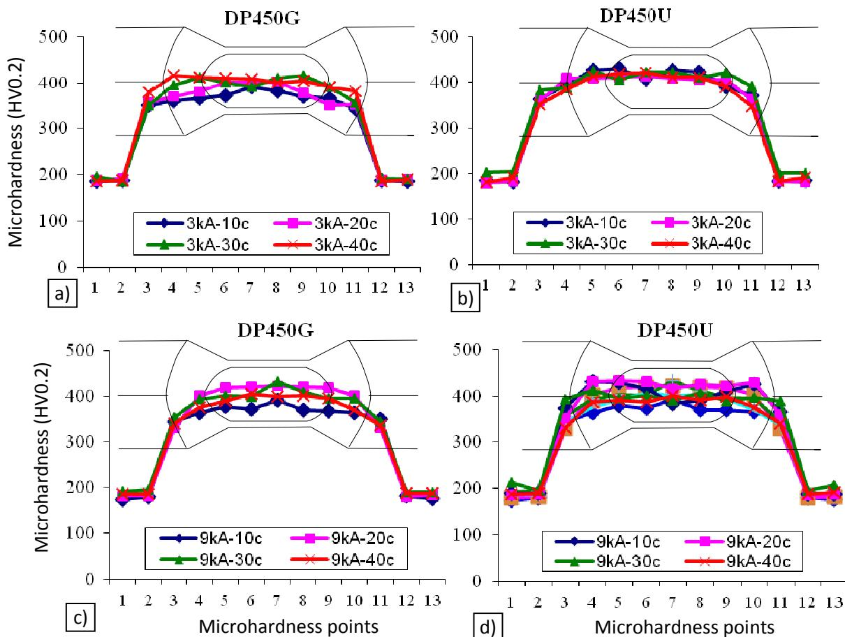
**Figure 3.** Micro-hardness values of DP450 steels welded by resistance spot welding at 10, 20, 30 and 40 cycles; (a) DP450G with 3 kA (b) DP450U 3 kA (c) DP450G 9 kA and (d) DP450U with 9 kA.
