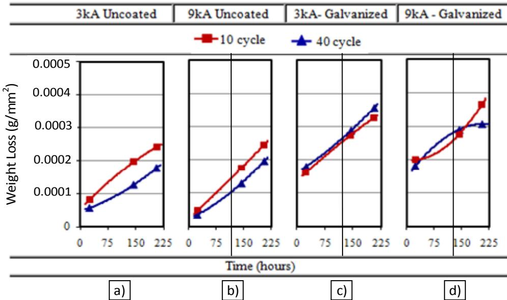
**Figure 5.** Change of weight loss in the welded specimens of the galvanised and uncoated steels.
