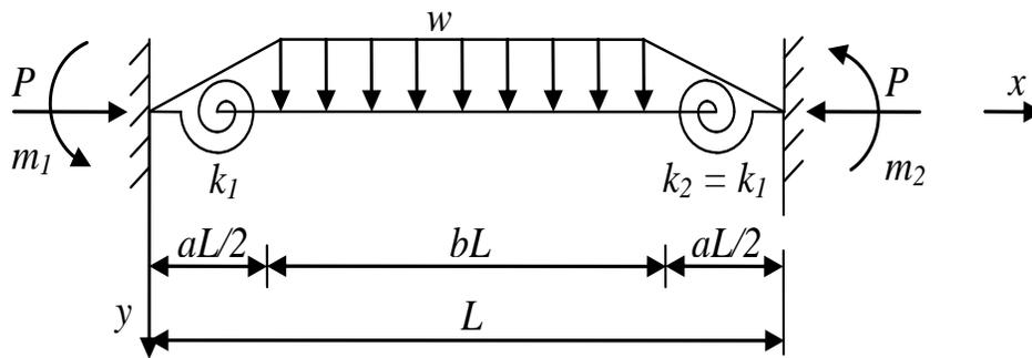
Figure 6. Symmetrical trapezoidal load.
