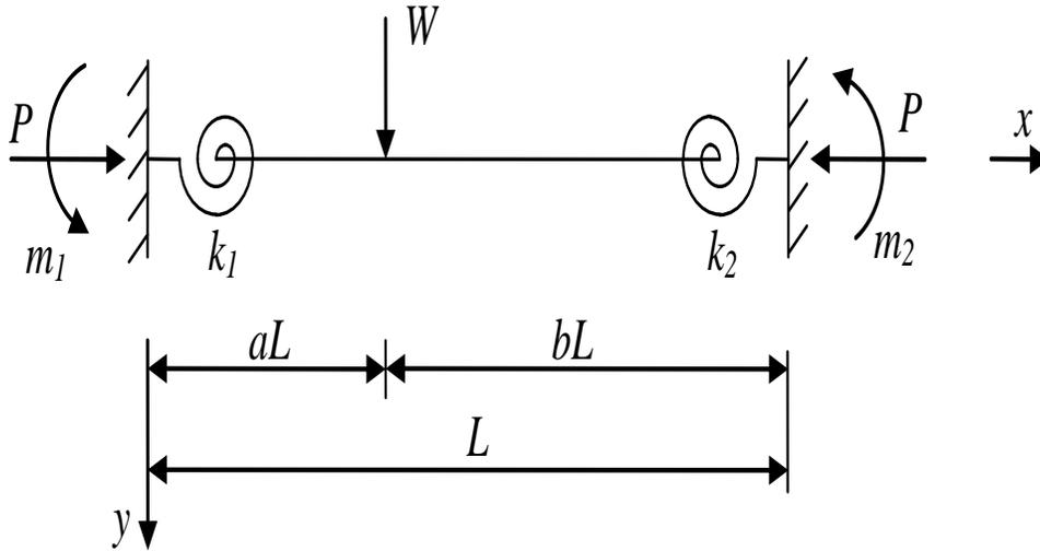
Figure 4. Single-point load.
