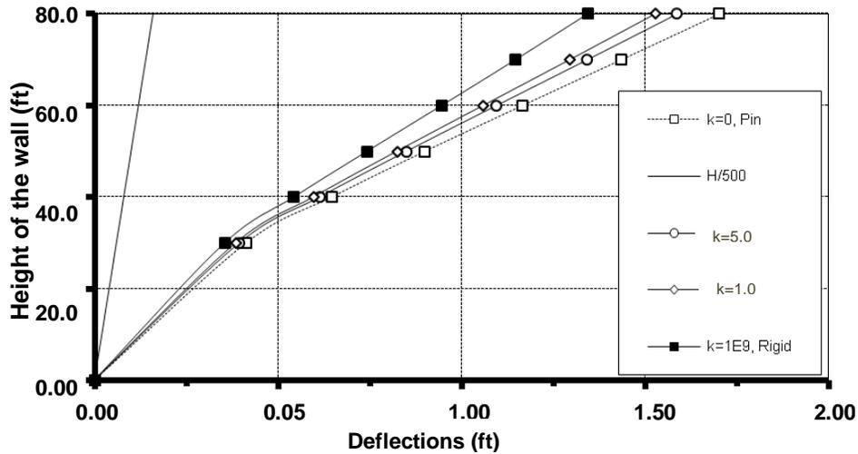
Figure 10. Lateral deflections at each floor level in the example problem with varying spring constants  $k$ .
