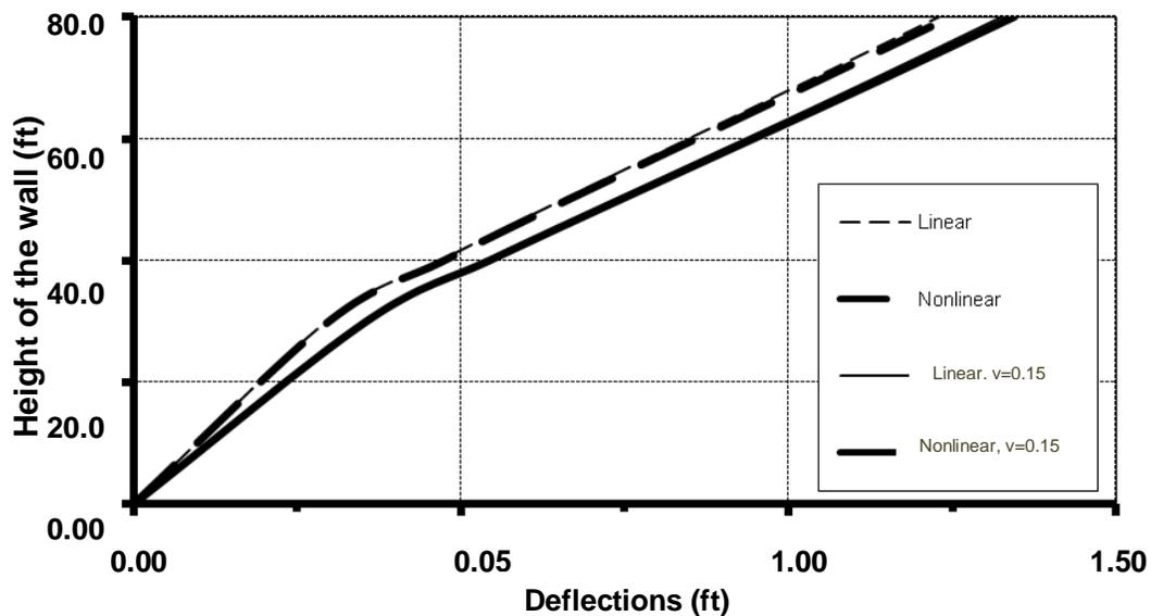
Figure 11. Lateral deflections at each floor level in the example problem with rigid connections.
