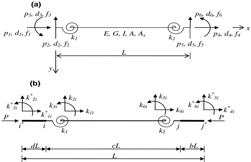
Figure 1. (a) Beam-column member model and (b) Beam-column member model with rigid end sections.
