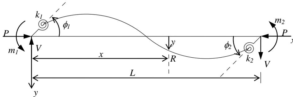
Figure 2. Directions and positive senses of various end properties.
