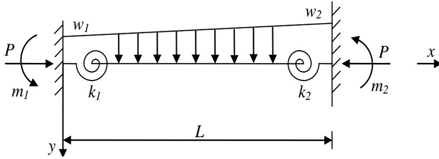
Figure 5. Linear variation of load.
