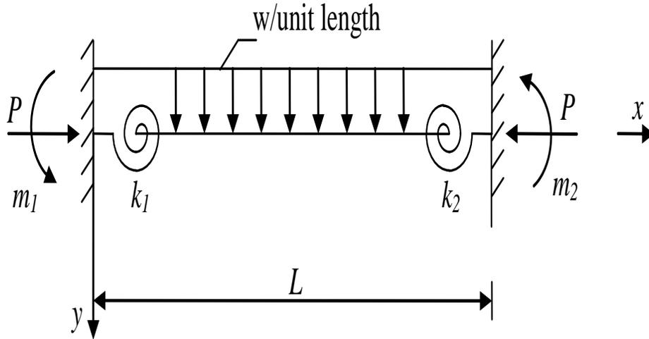
Figure 3. Uniformly distributed load.
