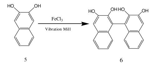
Scheme 3. Oxidative coupling of 2, 3-dihydroxy-1, 4-naphthylene in a vibration mill at 30 Hz.
