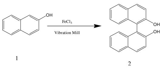
Scheme 1. Oxidative coupling of 2-Naphthol in a vibration mill.
