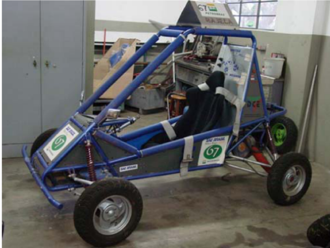
Figure 11. Electric vehicle type mini-baja Mini-baja has chassis single seat cage type with 1020 tubular steel frame, where length is 2 m, width is 1 m, height is 1.55 m, wheelbase is 1.70 m, and weight is around 205 kg. Its electric motor rated at 1.134 kW with maximum speed of 1,680 rpm, extruded in aluminium frame that significantly reduces its weight. Other characteristics are electronic speed controller and mechanical transmission of the drive system.
