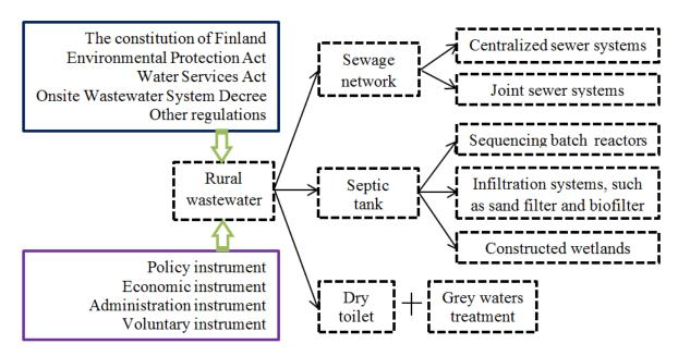
Figure 3. Finnish rural wastewater management and treatment technologies used in practice.
